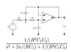
Using the above active filter blocks, design a Butterworth highpass filter with cutoff frequency of  $\omega_c = 2000 \text{ rad/s}$  and a pass-band gain of magnitude 34dB. If the gain must be below 0dB for frequencies below 500 rad/s, what is the minimum filter order? Specify all component values, using 10nF capacitors whenever possible without increasing the part count. (30)
