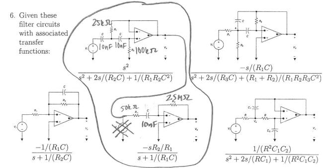
Using the above active filter blocks, design a Butterworth highpass filter with cutoff frequency of  $\omega_c = 2000 \text{ rad/s}$  and a pass-band gain of magnitude 34dB. If the gain must be below 0dB for frequencies below 500 rad/s, what is the minimum filter order? Specify all component values, using 10nF capacitors whenever possible without increasing the part count. (30)
