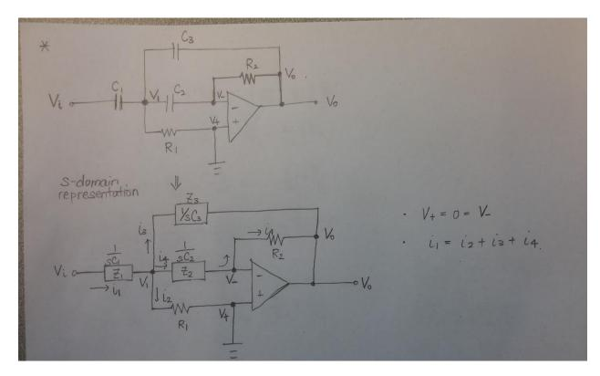
$$i_1 = \frac{V_i - V_1}{Z_1}, \ i_2 = \frac{V_1 - V_+}{R_1} = \frac{V_1}{R_1}, \ i_3 = \frac{V_1 - V_0}{Z_3}, \ i_4 = \frac{V_1 - V_-}{Z_2} = \frac{V_1}{Z_2} = \frac{V_- - V_0}{R_2} = \frac{-V_0}{R_2}$$
