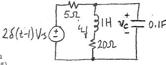
A filter is constructed using the circuit at the right.
