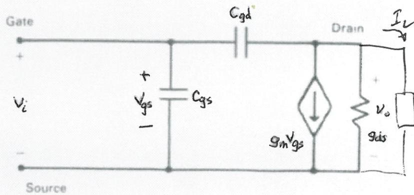
We can reduce this circuit to its Thevenin or Norton equivalent and power is maximized by making
