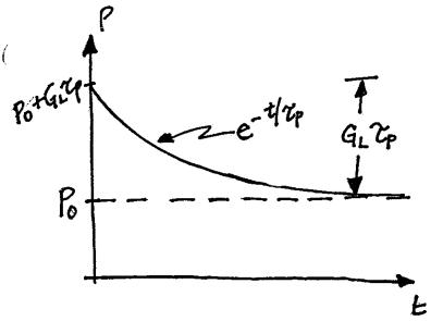
Note that both the electron and hole concentrations decay at the same rate. The excess minority carrier density is usually the important one in devices.
