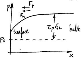
In that case, there is a net flow of carriers towards the surface (both  $h^+$  and  $e^-$  for charge neutrality and no net current).
