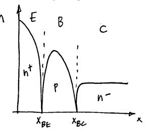
The impurity profile at left represents the positions of the fixed ionized dopant atoms.
