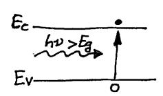
At any T > 0°K, some electrons gain enough energy to jump into the conduction band. This leaves behind a hole so that
