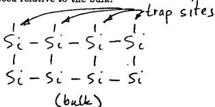
Incompletely bonded silicon atoms at the surface can provide efficient traps for recombination.
