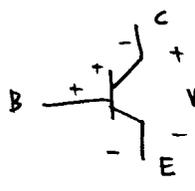
$V_{BE} > 0$  because  $I_B$  is positive.
