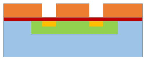
Step 6: Strip photoresist. Drive in the implanted boron;
