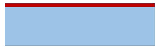
Step 2: Deposit, expose and develop photoresist; Use mask #1 to pattern the photoresist;
