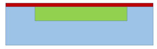
Step 4: Deposit, expose and develop photoresist; Use mask #2 to pattern the photoresist;
