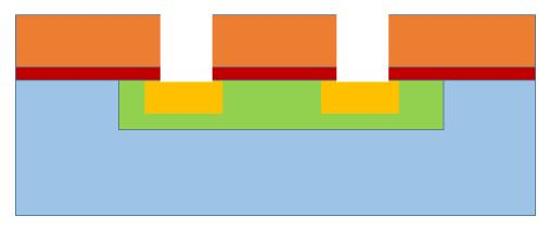
Step 10: Deposit, expose and develop photoresist; Use mask #3 to pattern the photoresist;
