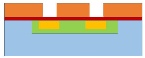
Step 9: Etch away the exposed oxide;
