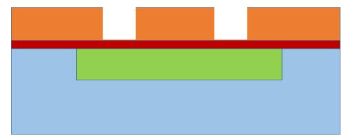
Step 5: Conduct p type implantion with boron;
