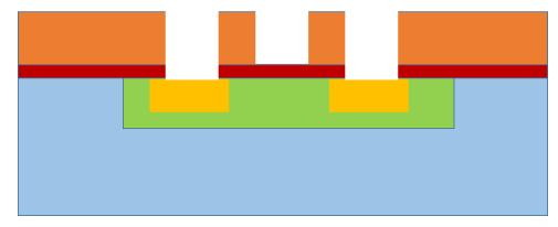
Step 11: Deposit metal and then lift off metal on top of photoresist
