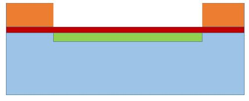
Step 4: Strip photoresist. Drive in the implanted phosphorus;
