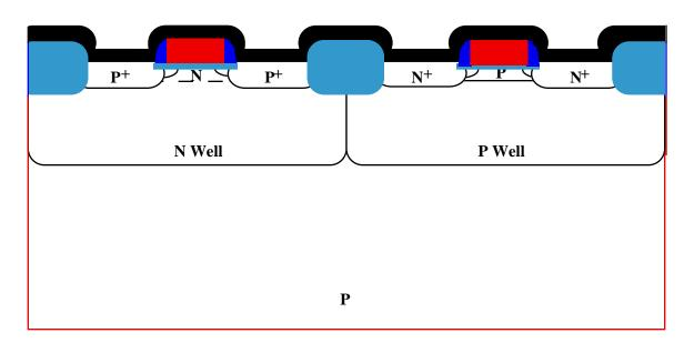
• Ti is deposited by sputtering (typically 1000 Å).
