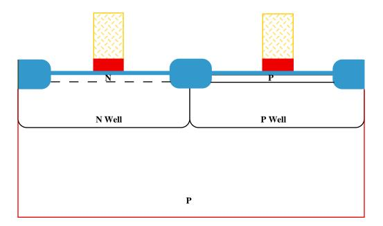
• Mask #6 is used to protect the MOS gates. The poly is plasma etched using an anisotropic etch.
