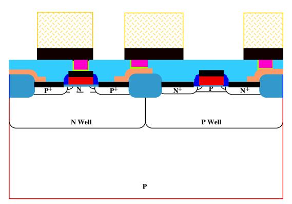
• Al is deposited on the wafer by sputtering. Mask #13 is used to pattern the Al and plasma etching is used to etch it.
