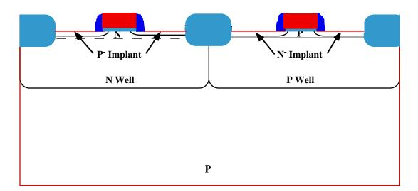
• Anisotropic etching leaves "sidewall spacers" along the edges of the poly gates.
