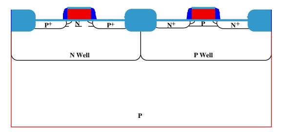
• A final high temperature anneal drives-in the junctions and repairs implant damage (typically 30 min @ 900 °C or 1 min RTA @ 1000 °C).
