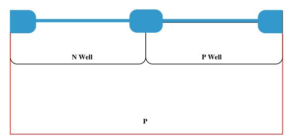
• A high temperature drive-in produces the "final" well depths and repairs implant damage. Typically 4-6 hours @ 1000 °C - 1100 °C or equivalent Dt.
