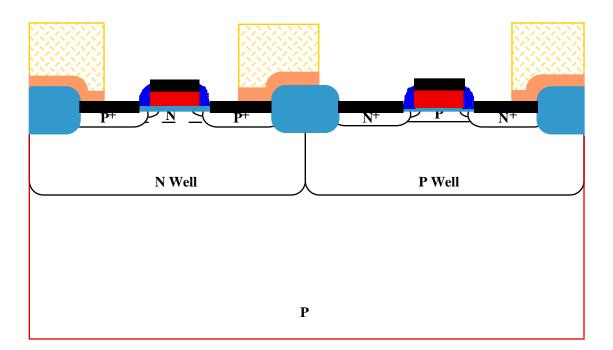
• Mask #11 is used to etch the TiN, forming local interconnects.
