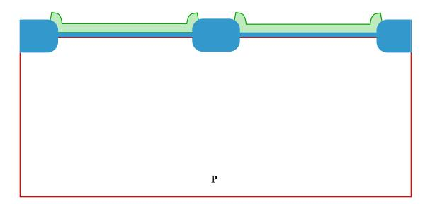
• Field oxide is grown using a LOCOS process. Typically 90 min @ 1000 °C in  $H_2O$  grows  $\approx 0.5 \ \mu m$ .
