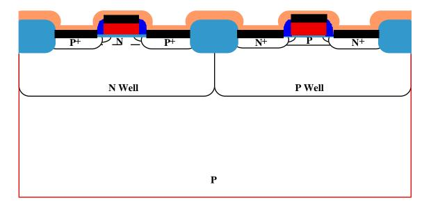
• The Ti is reacted in an N<sub>2</sub> ambient, forming TiSi<sub>2</sub> and TiN (typically 1 min @ 600 °C).
