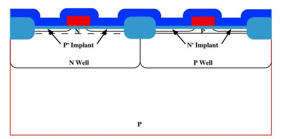
• A conformal layer of  $SiO_2$  is deposited (typically 0.5  $\mu$ m).
