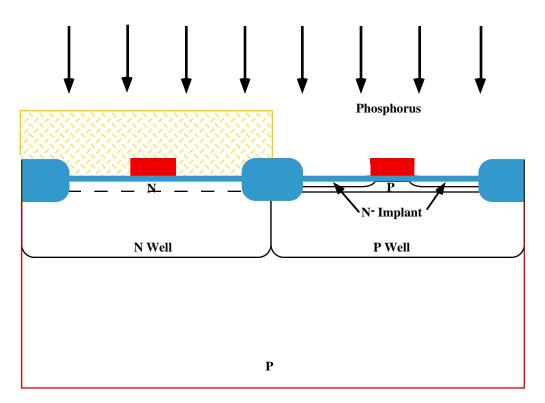
• Mask #7 protects the PMOS devices. A P<sup>+</sup> implant forms the LDD regions in the NMOS devices (typically  $5 \times 10^{13} \text{ cm}^{-2} @ 50 \text{ KeV}$ ).
