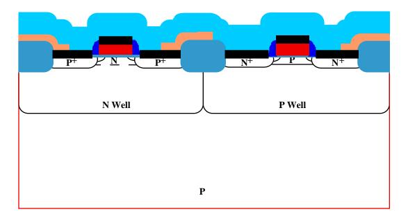
• A conformal layer of  $SiO_2$  is deposited by LPCVD (typically 1  $\mu$ m).
