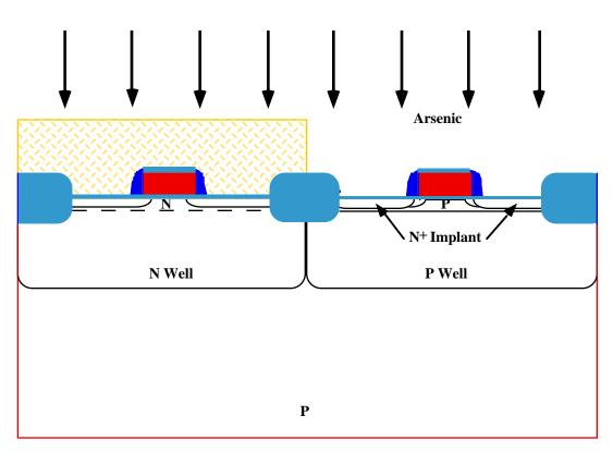
Mask #9 protects the PMOS devices, An As<sup>+</sup> implant forms the NMOS source and drain regions (typically 2-4 x 10<sup>15</sup> cm<sup>-2</sup> @ 75 KeV).
