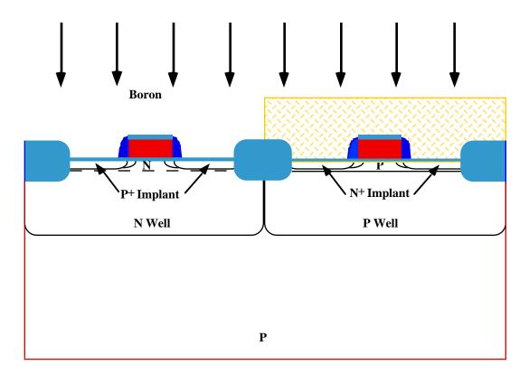
Mask #10 protects the NMOS devices, A B<sup>+</sup> implant forms the PMOS source and drain regions (typically 1-3 x 10<sup>15</sup> cm<sup>-2</sup> @ 50 KeV).
