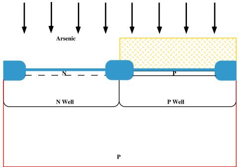
• Mask #5 is used to mask the NMOS devices. A  $V_{TH}$  adjust implant is done on the PMOS devices, typically 1-5 x  $10^{12}$  cm<sup>-2</sup> As<sup>+</sup> implant @ 75 - 100 KeV.
