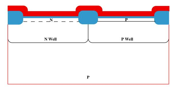
• Polysilicon is deposited by LPCVD (  $\approx 0.5 \ \mu m$ ). An unmasked P<sup>+</sup> or As<sup>+</sup> implant dopes the poly (typically 5 x 10<sup>15</sup> cm<sup>-2</sup>).
