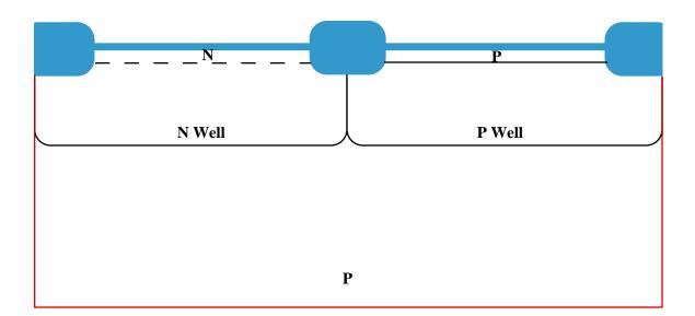
• The thin oxide over the active regions is stripped and a new gate oxide grown, typically 50 - 100 Å, which could be grown in 1 - 2 hrs @ 800 °C in O<sub>2</sub>.
