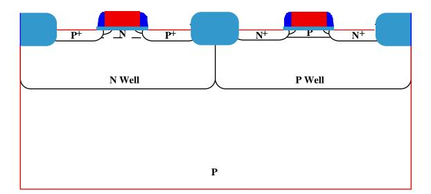
• An unmasked oxide etch allows contacts to Si and poly regions.
