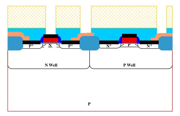
• Mask #12 is used to define the contact holes. The SiO<sub>2</sub> is etched.
