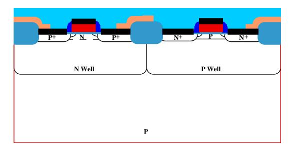
• CMP is used to planarize the wafer surface.
