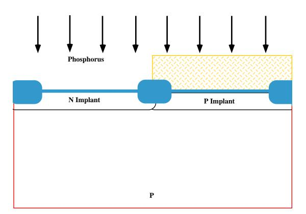
• Mask #3 blocks a P<sup>+</sup> implant to form the wells for the PMOS devices. Typically 10<sup>13</sup> cm<sup>-2</sup> @ 300<sup>+</sup> KeV.
