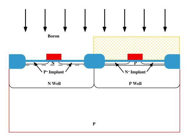
• Mask #8 protects the NMOS devices. A B<sup>+</sup> implant forms the LDD regions in the PMOS devices (typically  $5 \times 10^{13} \text{ cm}^{-2}$  @ 50 KeV).
