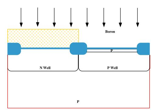
• Mask #4 is used to mask the PMOS devices. A  $V_{TH}$  adjust implant is done on the NMOS devices, typically a 1-5 x  $10^{12}$  cm<sup>-2</sup> B<sup>+</sup> implant @ 50 - 75 KeV.
