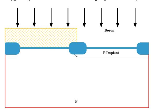
• Mask #2 blocks a B<sup>+</sup> implant to form the wells for the NMOS devices. Typically 10<sup>13</sup> cm<sup>-2</sup> @ 150-200 KeV.
