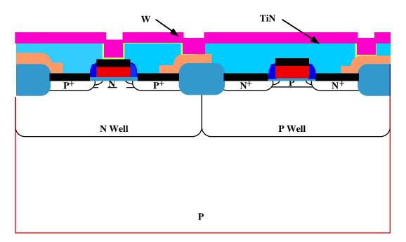
• A thin TiN barrier layer is deposited by sputtering (typically a few hundred Å), followed by W CVD deposition.
