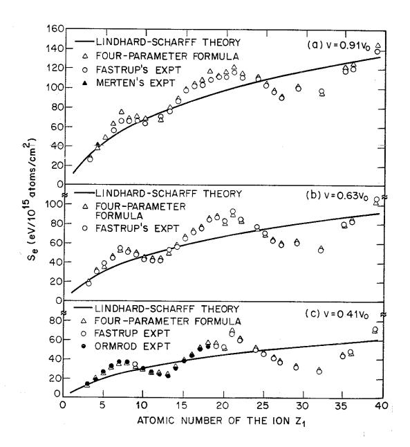
Electronic Stopping is generally considered inelastic because electrons that gain energy lose it immediately in the form of heat.
