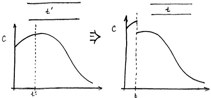
Although more complex to implement, the alternative, dose matching, does a better job of giving the correct distribution in the film. It takes advantage of the fact that the implant profile in the film is nearly independent of the underlying substrate (little difference in backscattering).
