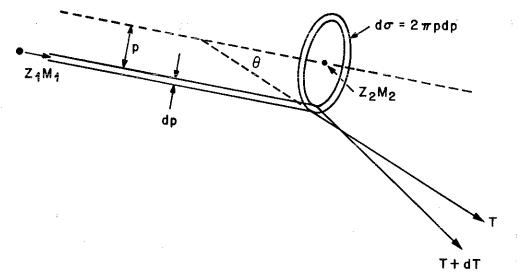
Scattering probabilities increase as  $d\sigma$  increases.  $d\sigma$  increases with increasing p, but the magnitude or strength of the interaction decreases.
