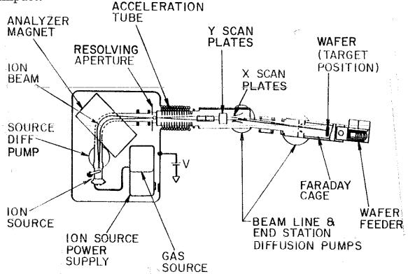
Gas Source: Provides desired impurities to be ionized. Extremely high purity is not essential since mass separation is usually done anyway.
