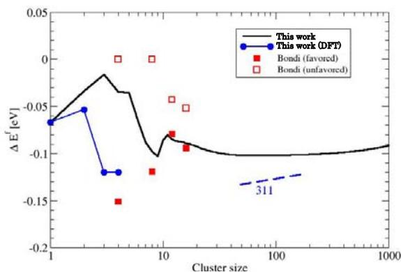
Figure 2: The strain-induced change in cluster formation energy for strained Si on 20%Ge, expressed as average energy per interstitial
