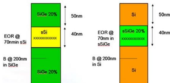
Figure 1: Schematic illustration of strained-Si and strained-SiGe structures used in experiments
